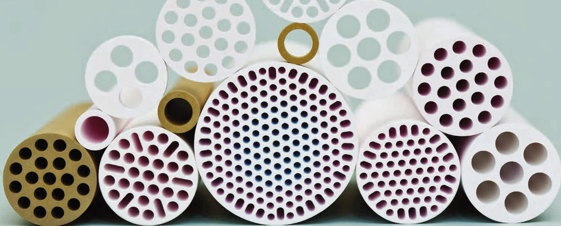
Ceramic filtration membranes. (Fraunhofer IKTS)
