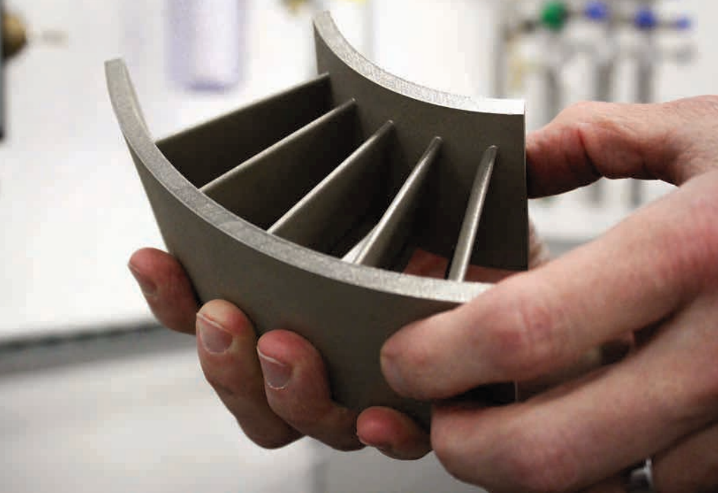
Hebert holds additively manufactured samples for R&D that emulate real-world component designs.
