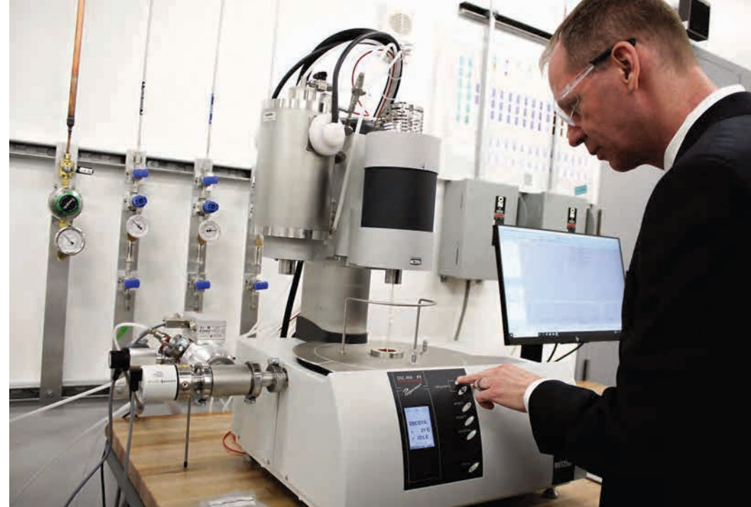
Hebert works with equipment to determine melting points and other thermodynamic properties at temperatures up to about 3,000 degrees Fahrenheit.
